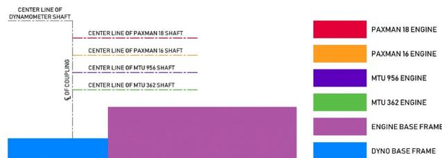
Figure-3 Engine-Dyno shafts relative height representation
