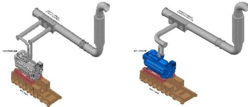
Figure 5: Exhaust trunking for Paxman V16 & V18 (left) and MTU 956 & 362 (right)
